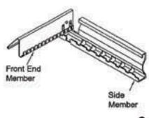
Install front end member as described in step 3. NOTE: If stabilizer is needed, hook stabilizer loop around one of the center teeth of the rear end member and pull to the front member where it hooks around corresponding teeth.
