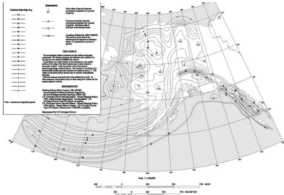
Figure 2.6.3-4 Maximum Considered Earthquake Ground Motion for Alaska of 1.0 sec Spectral Response Acceleration (5% of Critical Damping), Site Class B
