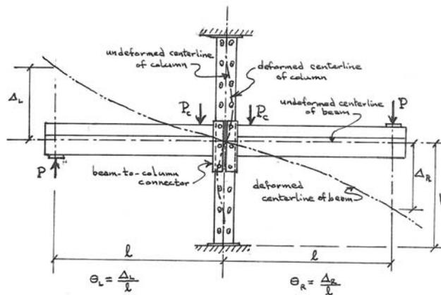
Figure 9.6.5-1 Test Set Up
