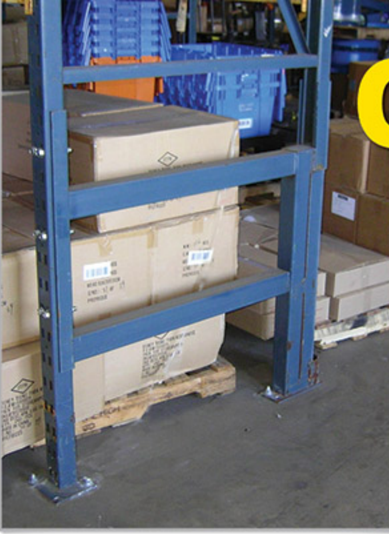
Straight leg - bolted repair kit
