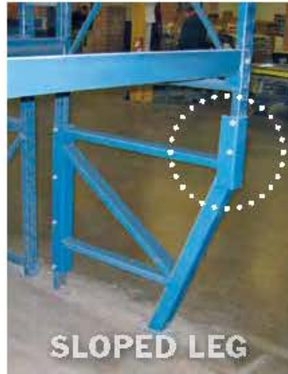
Bolt-on sloped leg option gets the upright out of the forklift traffic path to prevent repetitive damage.
