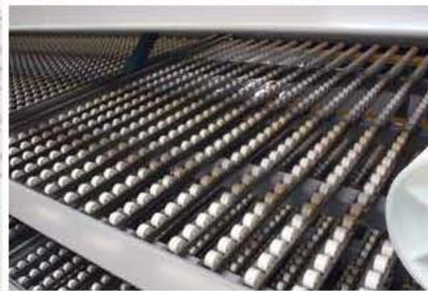
Carton Trax: steel axle carton flow with UPICK knock-down modular shelves.
