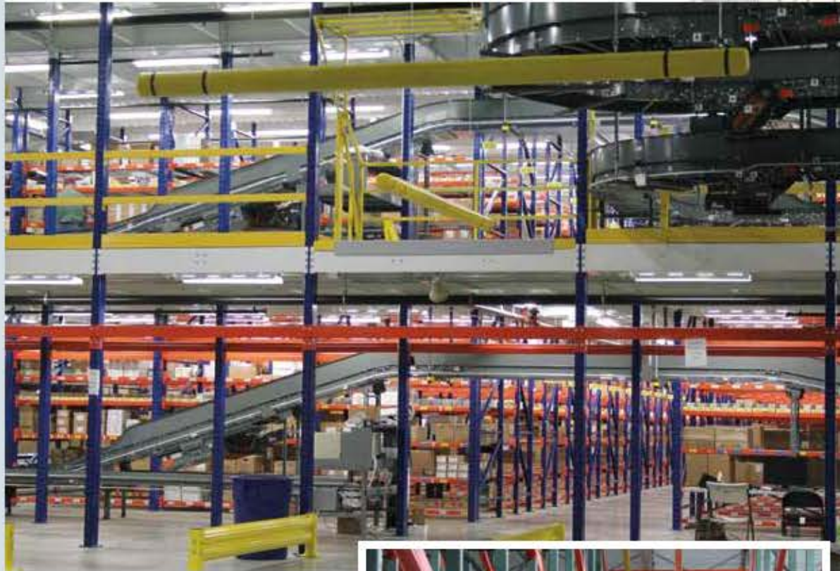
Conveyors run through multi-level rack-supported systems for product sortation
