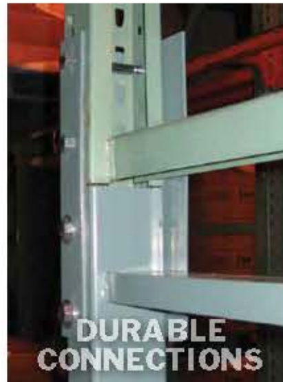
Bolt-on sloped leg option gets the upright out of the forklift traffic path to prevent repetitive damage.
