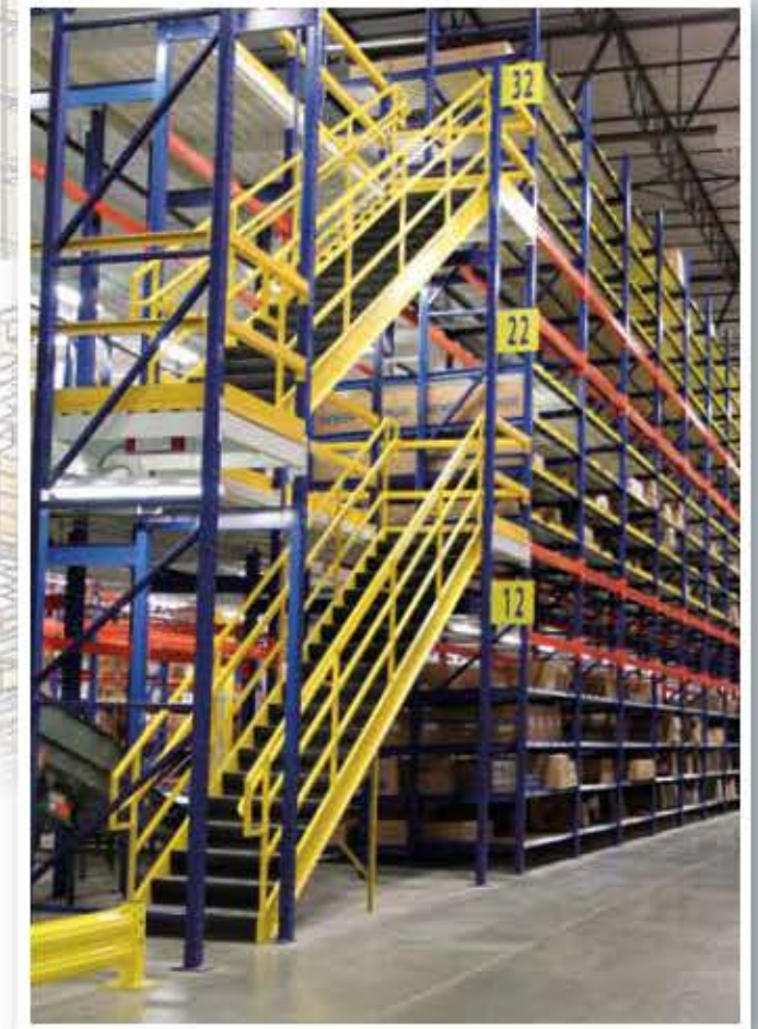
Integrated stairs and work platforms help product breakdown from pallet to carton to piece for easy order fulfillment.
