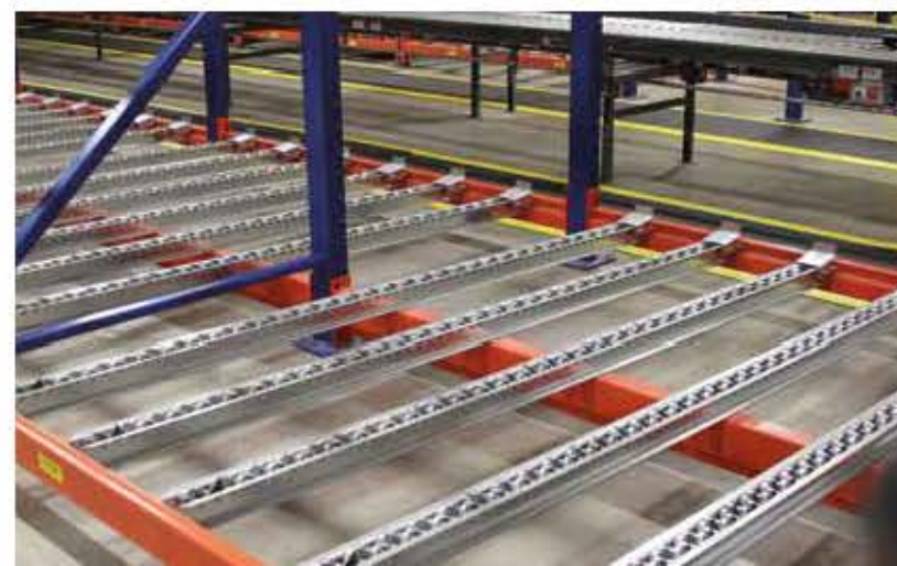
Pallet Flow used in pick module application with carton flow above
