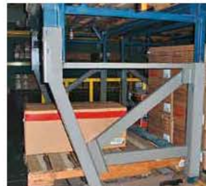
Bolt-on sloped leg option gets the upright out of the forklift traffic path to prevent repetitive damage.
