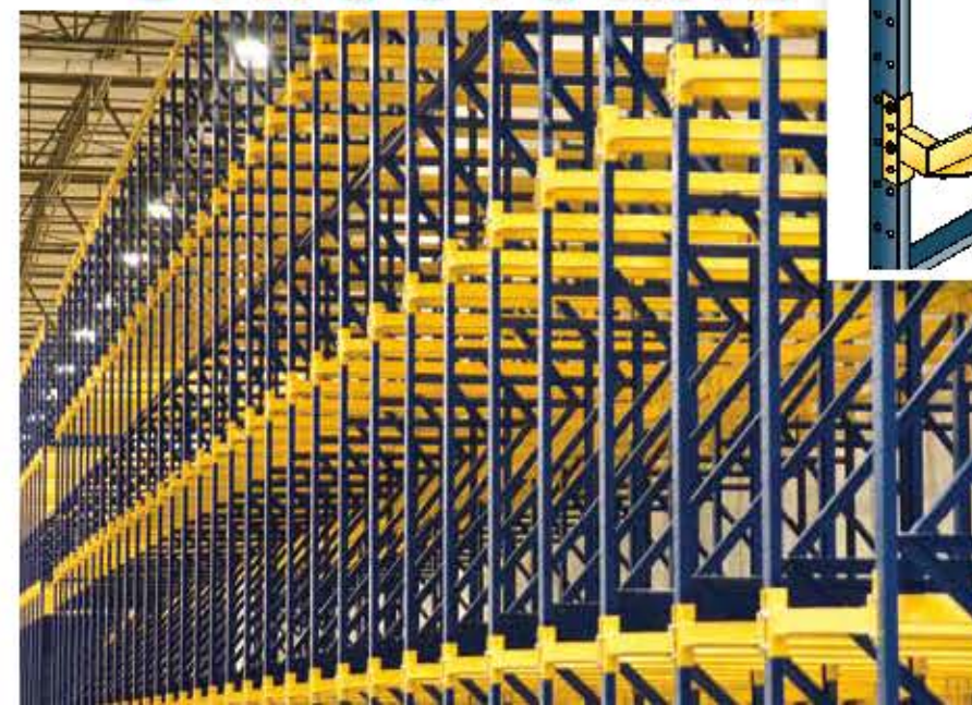
Drive-In Rail with Space Saver Arm for easier placement of pallets (shown with rounded and flared entry rail)
