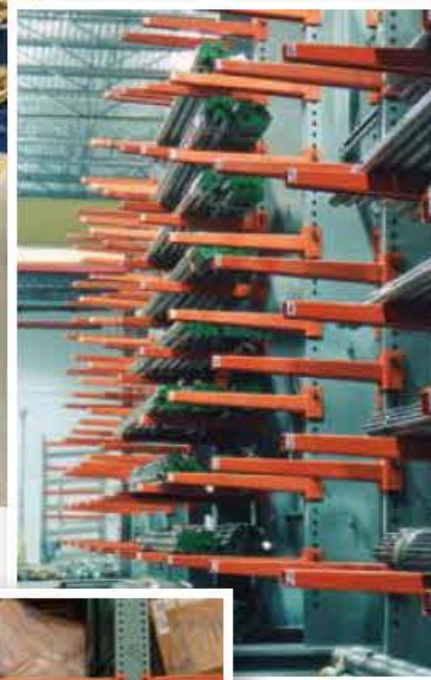
Pipe storage cantilever
