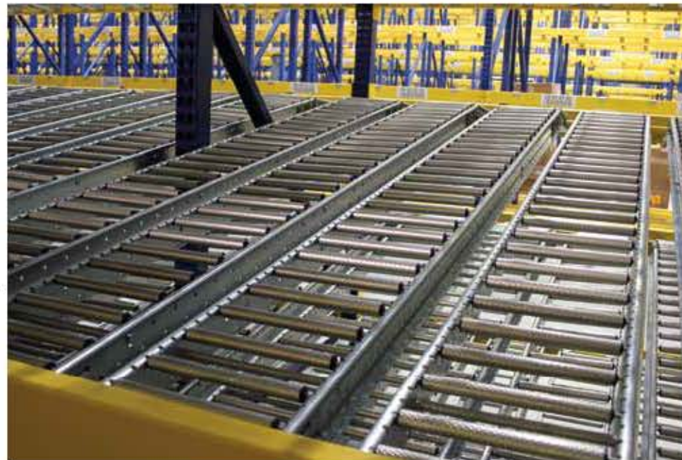
RhinoDeck with 11" high galvanized steel side channels will drop into any existing carton flow system with no hardware or hanger brackets required.
