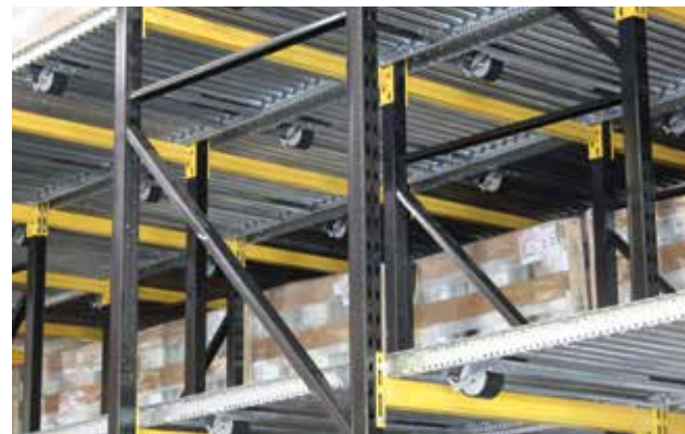
Factory-installed brakes are used for speed control in deep lane wide-roller systems.
