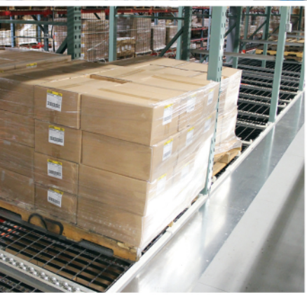
Pallets rest against pallet stop
