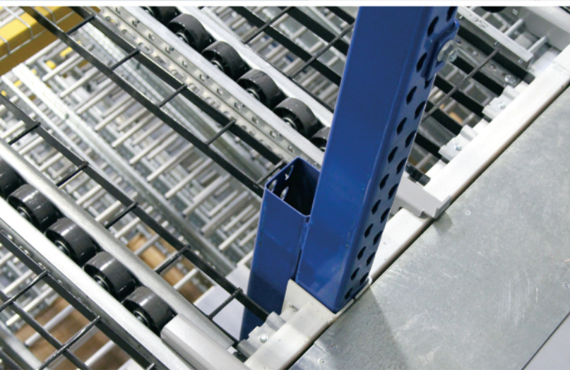
Pallet flow rails are notched to rest on the step of the beam for a lower profile that protects ends of flow rail
