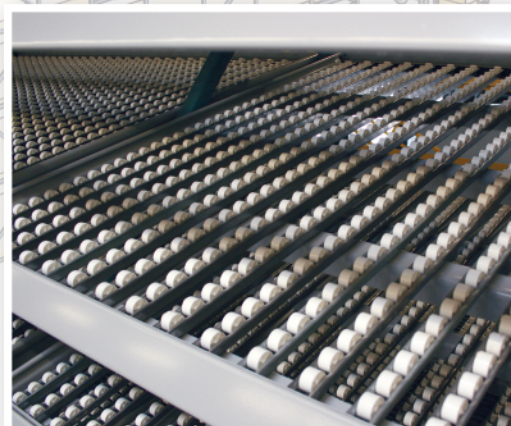
Carton Trax steel axle carton flow with UPICK knock-down modular shelves.
